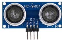
Fig 5: Ultrasonic Sensor HC-SR04 used in the system
